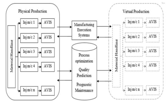
Figure 6. Digital Twin of injection molding process. (Injection m/c: injection molding machine; AVIS: automated visual inspection system)
